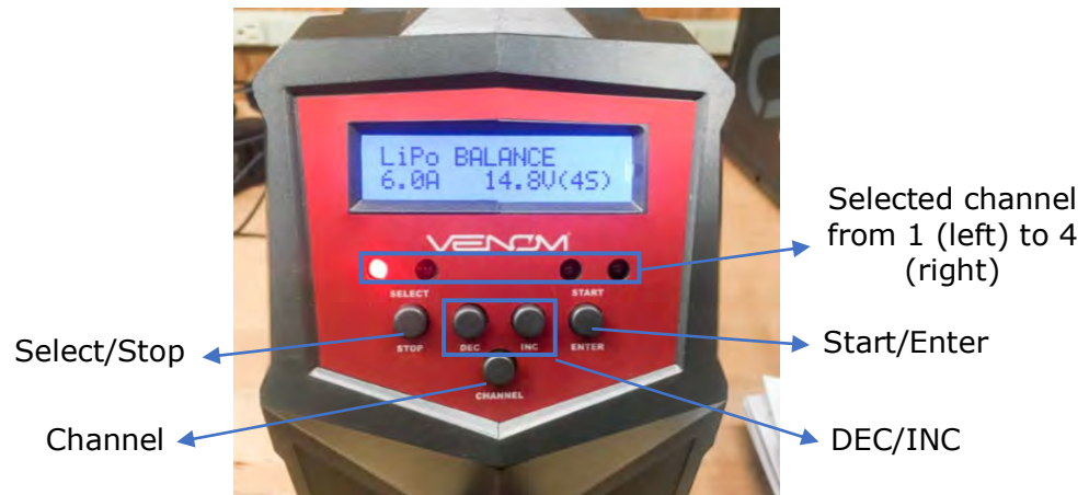
Figure 6: Venom PROQUAD charger displaying the right settings for the 4S batteries and meaning of the different buttons
