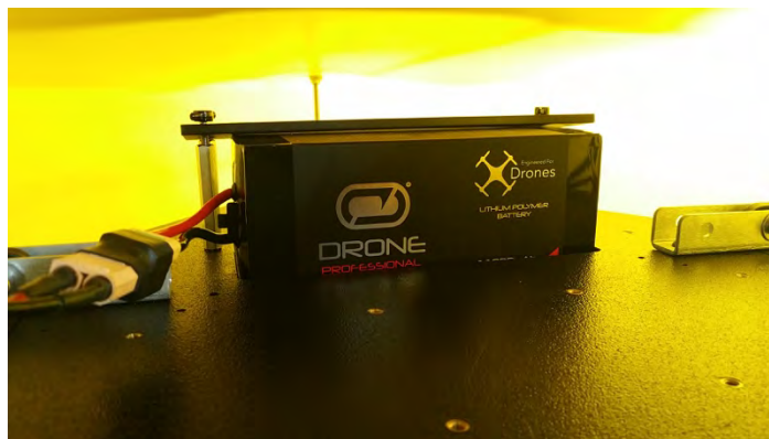
Figure 13: 6S batteries panel on the bow of the EchoBoat
