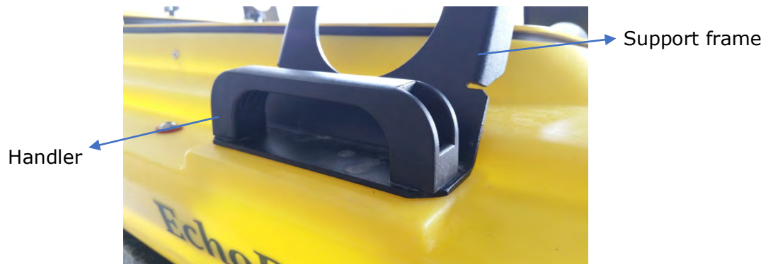
Figure 15: Support frame installation on the EchoBoat
