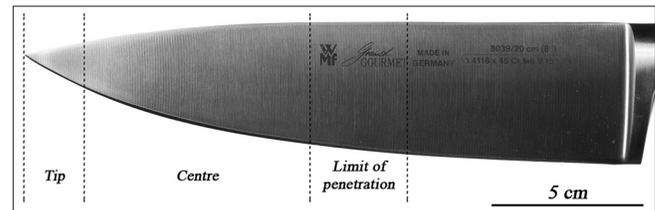
**Figure 3:** First segmentations of the blade (chef's knife): The tip, the centre and the limit of penetration
