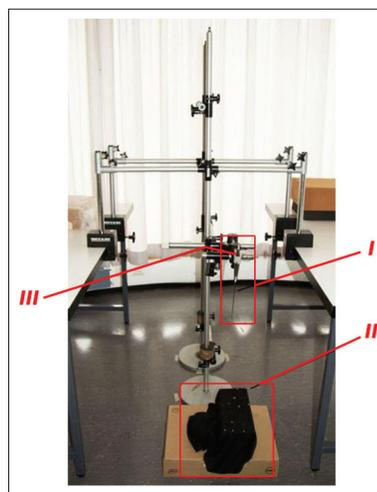
**Figure 2:** Apparatus used for the stabbing simulations with the designation of the knife (I), The garment (II) and the movable part (III)
