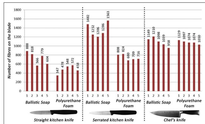
**Figure 5:** Number of fibres from the pyjama recovered in each simulation (simple transfer set)
