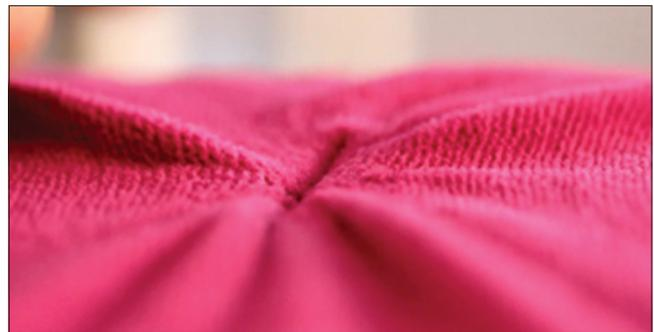
Figure 7: Interaction between the pyjama and the ballistic soap simulant after the removal of the blade
