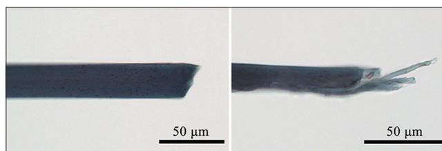
**Figure 11:** Extremities of a cut (left) and a torn (right) polyester fibre from the black shirt. The cut fibre presents a sharp extremity, while the torn one is frayed
