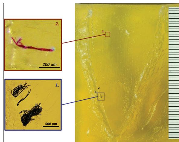
**Figure 16:** Stab damage (inside the ballistic soap) created by the chef's knife during the stabbing sequence pyjama → shirt (simulations number 5 and number 6). Tufts originating from the black shirt (1) and fibres from the pyjama (2) were recovered
