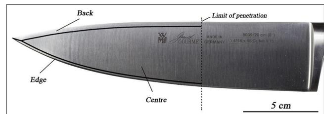
**Figure 4:** Second segmentation of the blade (chef's knife): The cutting edge, the centre and the back of the blade
