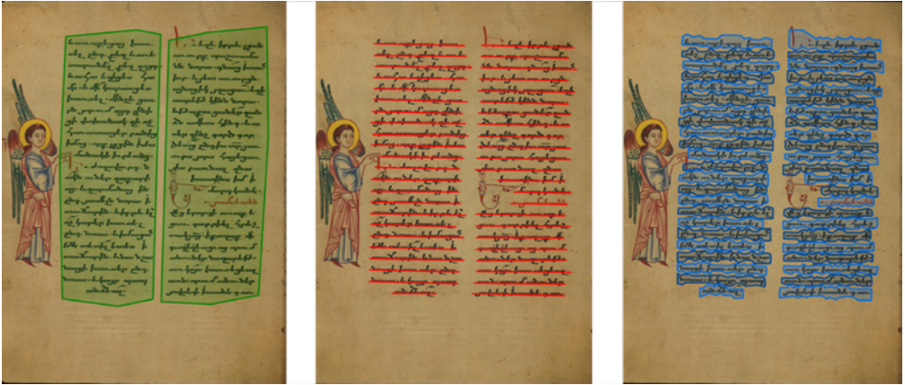
Figure 4a (i) Layout analysis with text-regions identification, (ii) line detection, and (iii) line extraction (MS W541, f. 114v). The user keeps control over each step on Calfa Vision in order to ensure high recognition rates
