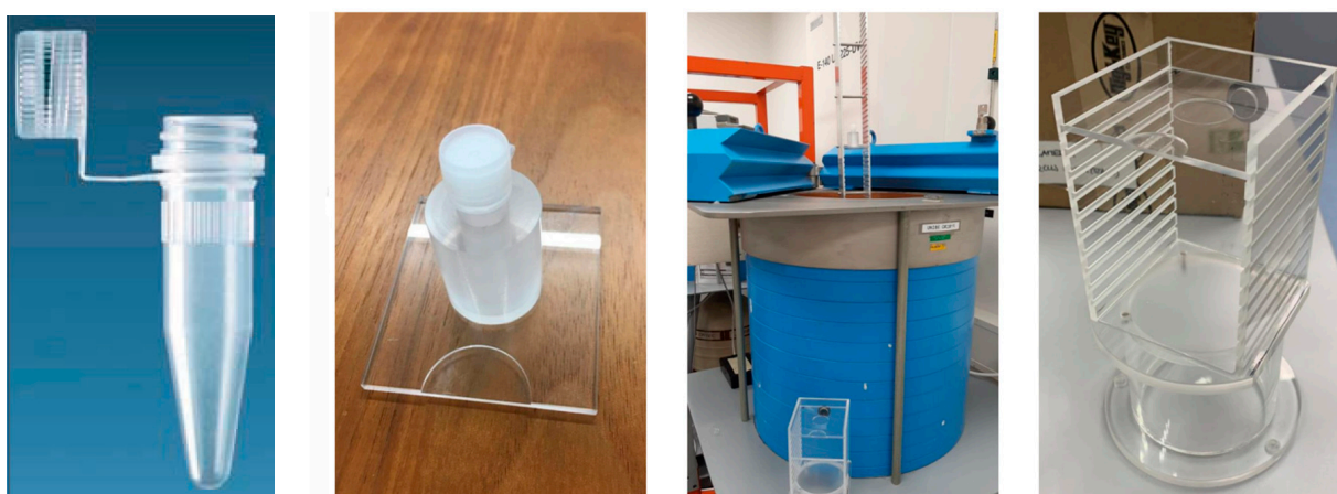
Figure 4. Images of the Eppendorf positioning system at the University of Bern. From left to right: Eppendorf vial, Eppendorf holder, detector enclosure, and positioning device.
