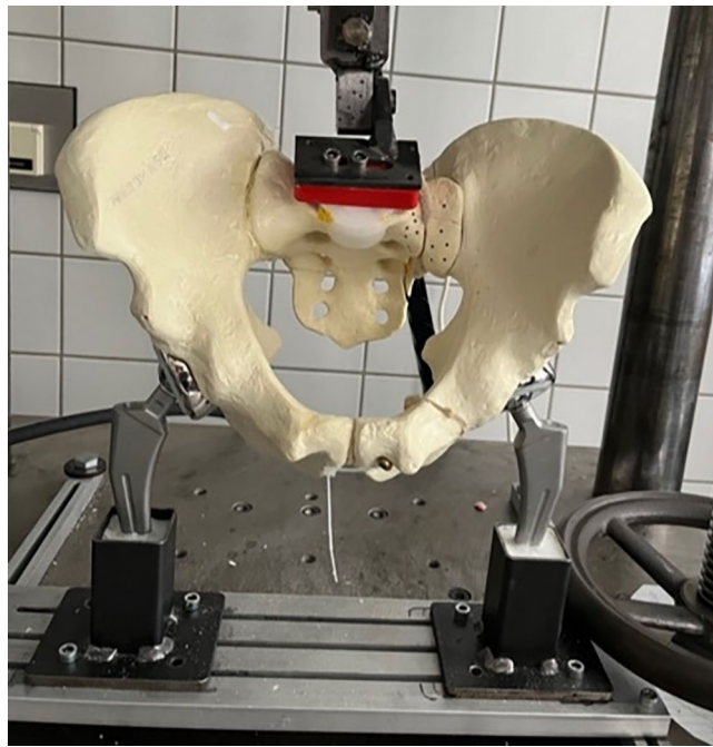
Fig. 3. Sawbone specimen (group SI+) set of two bipolar hip prosthesis and attached to the lever arm of the test machine at the endplate of S1.
