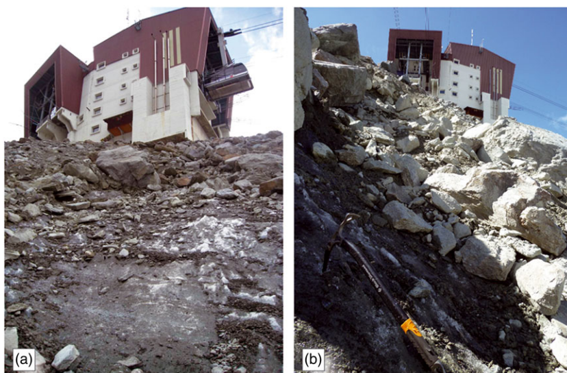
FIGURE 3 Massive ice with the presence of air bubbles (lower half on ph. (a) and bottom left on ph. (b)) revealed in landslide starting zones. (a) Starting zone of the two juxtaposed landslides of 1,138 ± 47 m 3 (see Figure 2.1d; photo: 5 October 2009); (b) northern margin of the starting zone of the 270 ± 12 m 3 landslide (see Figure 2.2f; photo: 30 August 2011) [Colour figure can be viewed at wileyonlinelibrary.com ]
