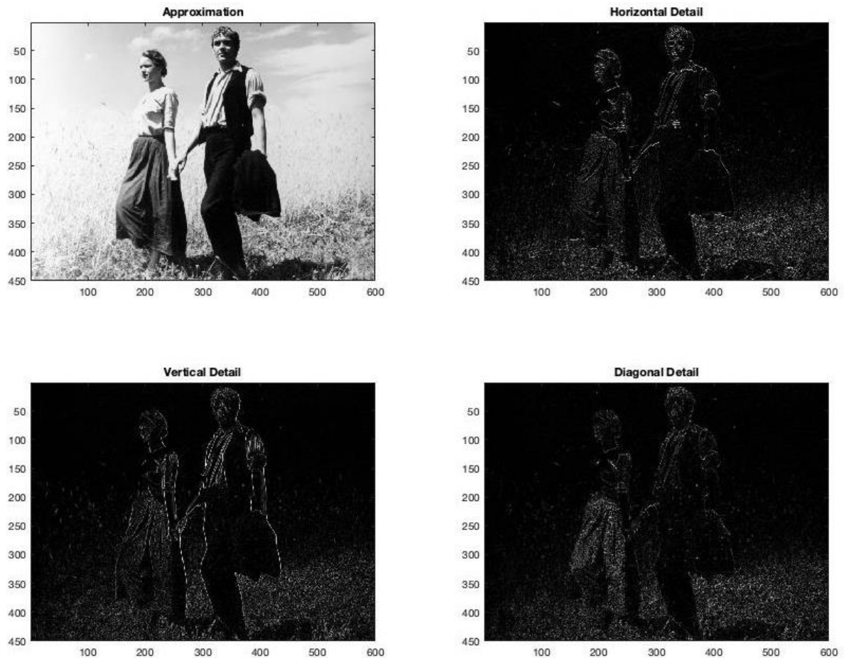
Figure 33 Wavelet coefficients for a digitised image of Romeo und Julia auf dem Dorfe (Hans Trommer, Valérien Schmidely, Switzerland, 1941, digitised in 4K). Original image courtesy of Cinémathèque suisse. Created by MATLAB coding.
