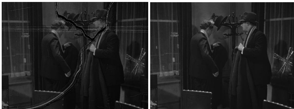
Figure 41 A tear removed during the 2013 restoration of La Chienne (Jean Renoir, 1931), as presented at Il Cinema Ritrovato Festival. Having received 70'000 euros from CNC, this restoration was conducted in the laboratory Digimage 40 and included rather complex operations of image restoration. 41
