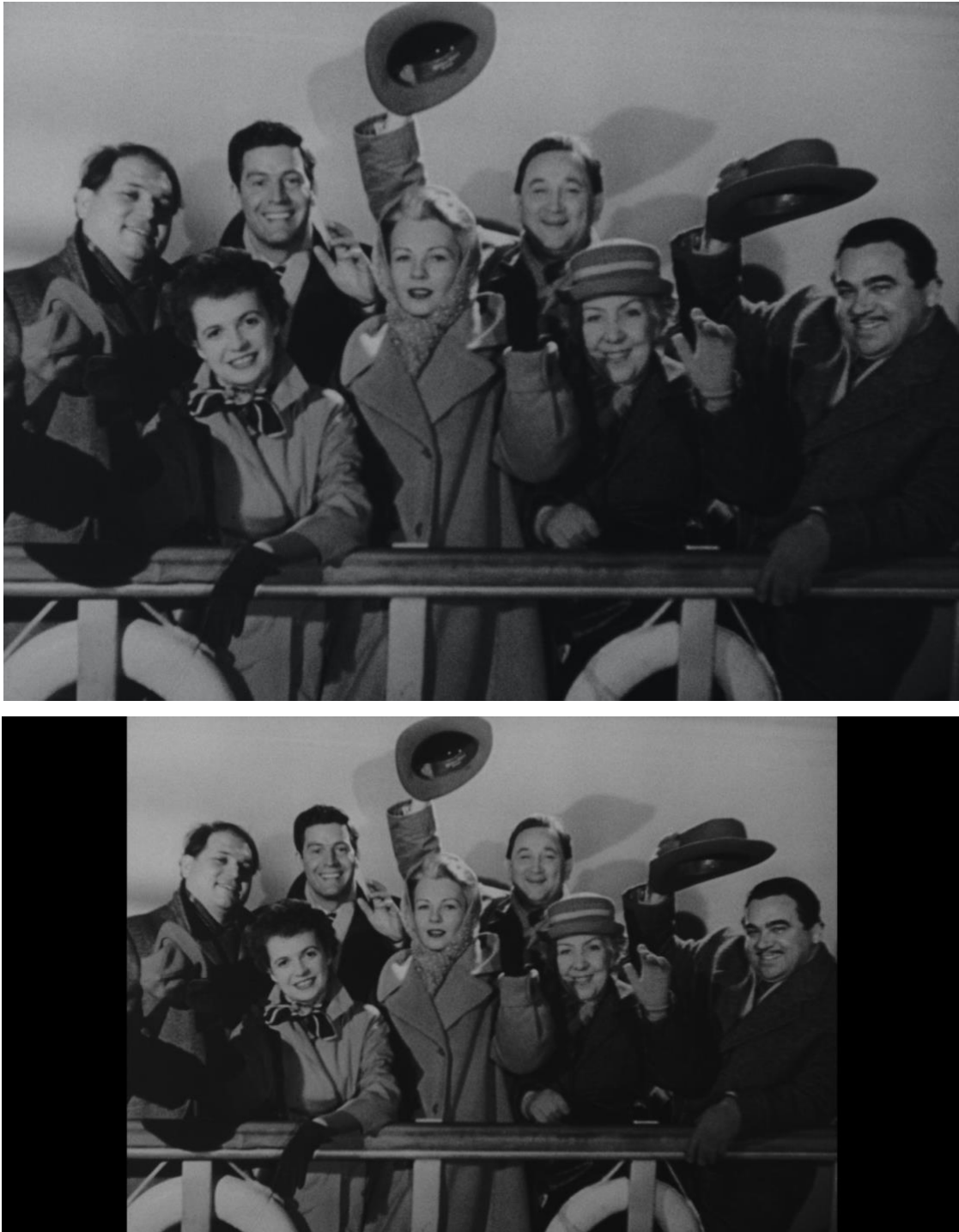
Figure 39 The dimensions of the 4K picture on top, in 1:1.37 aspect ratio, are 4096x2988. When the image is packaged into DCP, it needs to fit into the aspect ratio of 3996x2160. As seen in the bottom image, the height is therefore reduced from 2988 to 2160 pixels, and the DCP width of 3996, which is too big for the new image dimension of 2960 pixels, is filled on the sides by pillarboxes. Simply put, the image is described with a smaller number of pixels. This digitised frame comes from the 4K restoration of Venus vom Tivoli (Leonard Steckel, Switzerland, 1952). Courtesy of Cinémathèque suisse.
