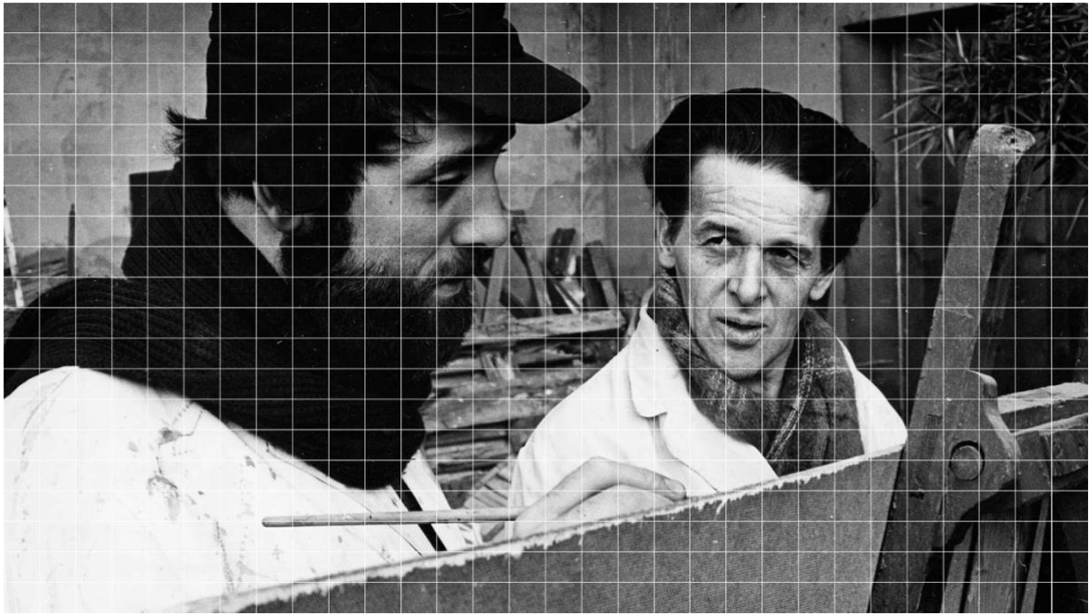
Figure 8 An example of how a grid of pixels is superimposed on a (digitised) photochemical image. Original photo courtesy of Cinémathèque suisse. The smaller the surface of each pixel, the more accurate the sampling.
