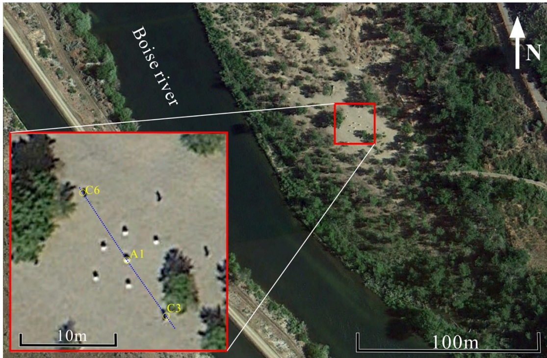
Figure 7. Location of BHRS wellfield in relation to the Boise River. The dashed blue line joining wells C6, A1, and C3 corresponds to the considered surface-based GPR reflection survey.
