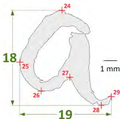
Figure 16 - Example of distance measurements (distances 18 and 19) between two coordinates.
