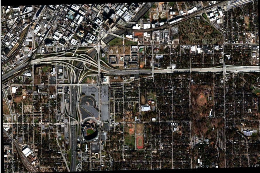
(a) True color composite (RGB: bands 5-3-2) of the image acquired at -8.5^\circ off-nadir (most nadiral image, i.e. image #7).
