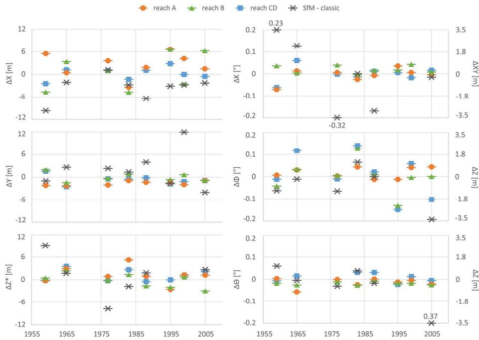
Figure 7 Adjustment of exterior parameters per reach with respect to deviation in bundle adjustment between SfM and classical photogrammetry (when they plot outside the y axis range, values are given - Table 4). \*For  $\Delta Z$  the values are corrected for focal length adjustment using the linear relation in Figure 2. The second y-axis for the orientation parameters gives the potential error in meters in a 1000 m reach.
