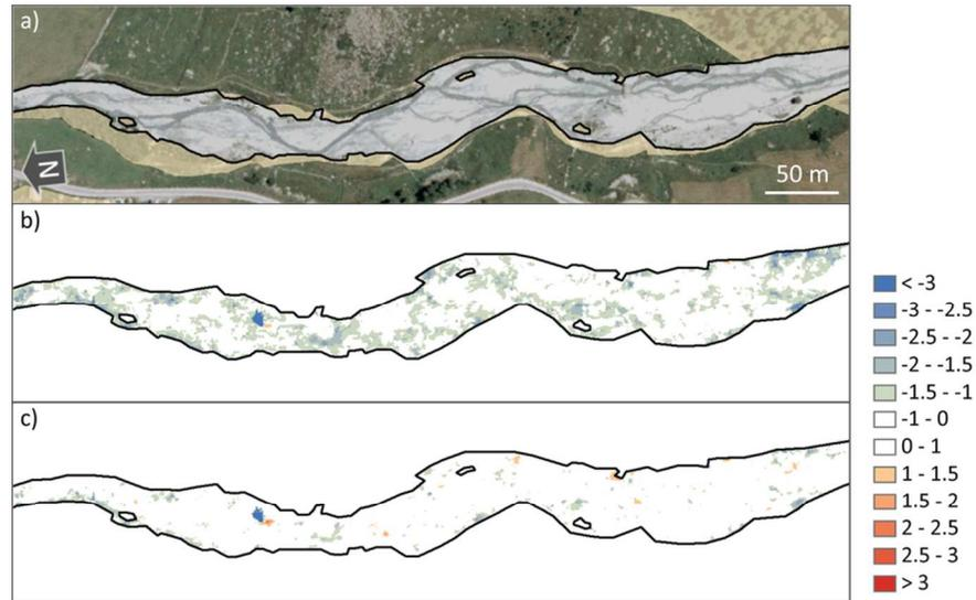
Figure 5 a) 2005 Orthoimage of the main section of reach C and stable zones (non-stable river flood plain and forested areas are shaded), b) 2005-2010 DoD before and c) after point cloud registration (blue is erosion, red is deposition). Limit of detection (95% certainty) is  $\sim 1\text{m}$ .
