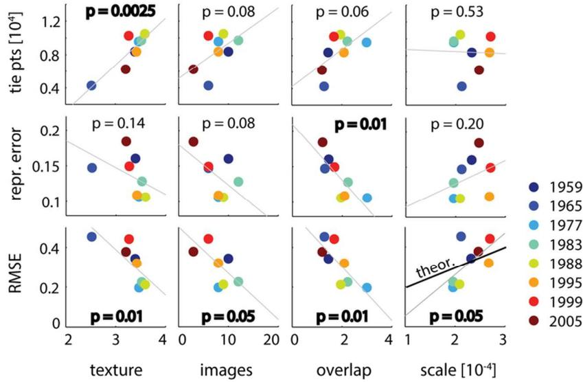
Figure 4 Scatter plots of image acquisition parameters, texture (entropy), images, image overlap and scale, vs. bundle adjustment parameters, tie points, reprojection error and RMSE. Plots include p values for Pearson's R linear correlation. Theoretical precision as a function of scale is plotted based on a 14  $\mu\text{m}$  resolution (1959 and 1965 have a 21  $\mu\text{m}$  resolution and therefore plot above the theoretical precision).
