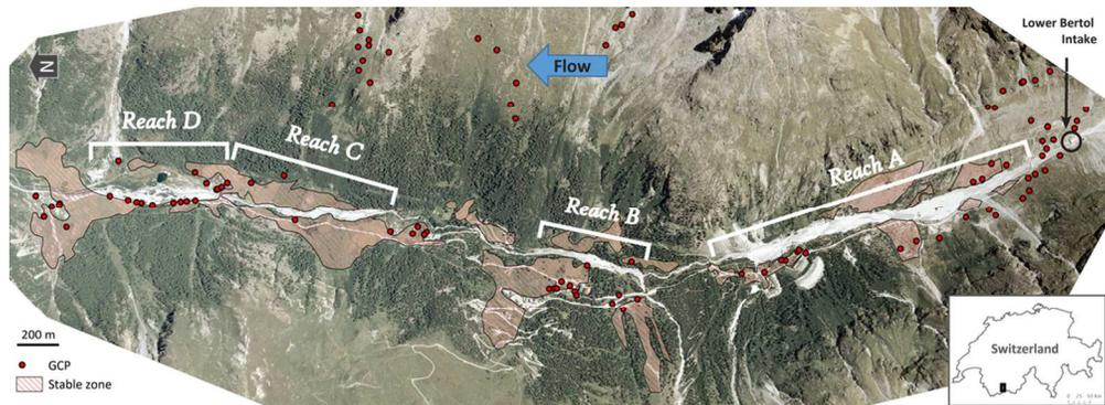
Figure 1 Orthoimage (2005) giving an overview of the sedimentation reaches in the Borgne d'Arolla River, Switzerland. GCPs and stable zones used for referencing and registration are shown.
