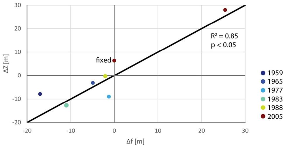
Figure 2 Relation between flying height difference ( $\Delta Z$ ) and the altitude difference that results from a change in focal length ( $\Delta f$ ) with respect to the calibrated value. Note that the line and statistics, Pearson's  $R^2$  and (significant) p value, follow a 1:1 relation and not a fitted regression line.
