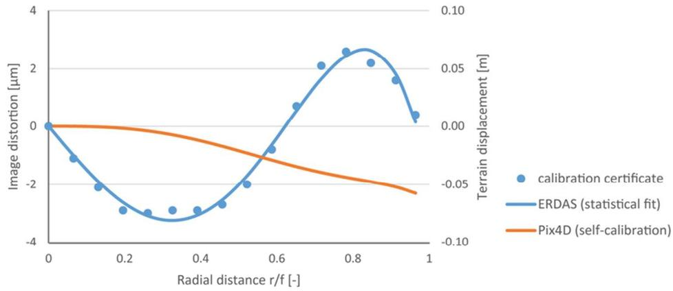
Figure 3 Radial distortion of the image and the related displacement in the terrain for the year with the largest calibrated distortion (2005). The ERDAS curve was statistically fitted using the measured deviations from the calibration certificate. The Pix4D curve was derived through self-calibration based on the images.
