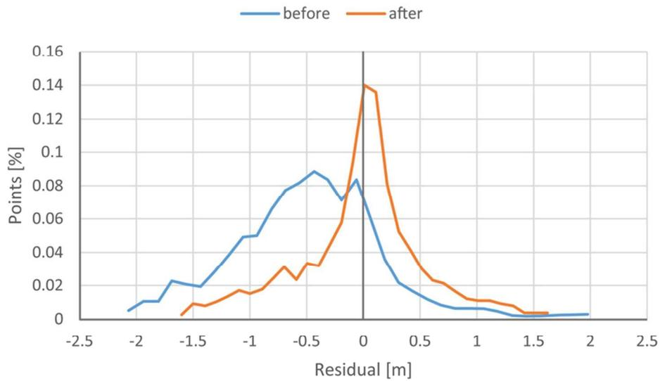
Figure 6 Normalised distribution of residual point distance between the stable zones in 2005 and 2010 for reach CD before and after registration.
