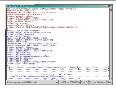
**Figure 2** Ethereal used to reconstruct one TCP stream in a peer-to-peer file exchange. The HTTP GET request from one KaZaA client is shown at the top of the screen and the corresponding response from the other KaZaA client is shown on the lower portion of the screen.
