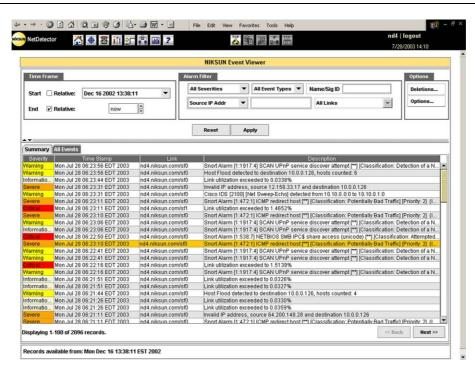
**Figure 6** Snort Alerts displayed in NetDetector's Event Viewer. NetDetector's Snort feature can operate in real-time or on stored data for post-event analysis.
