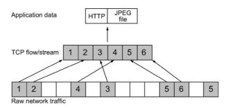
**Figure 1** A conceptual representation of packets in network traffic relating to a single flow being extracted and reconstituted to obtain the data they carry.
