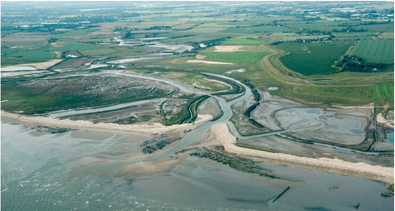
Aerial view of managed realignment at low tide - Photo credit: UK Environment Agency
