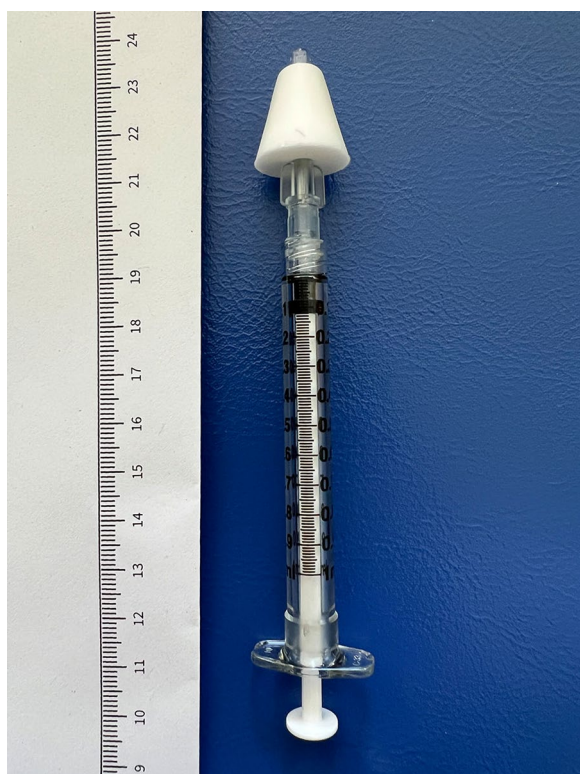
Fig. 1 Syringe (1 ml) with screw-on atomiser as used in this study
