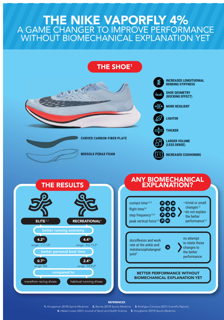
Figure 1. Infographic summarising the specificities of the Nike Vaporfly 4% running shoe, reporting the observed improvements in running economy and personal best time, and pointing out the absence of any biomechanical explanation to the better performance yet.
