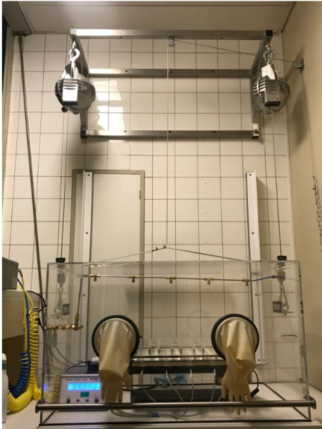
**Figure 1: Hypoxic setup.** The treadmill is placed inside the homemade glovebox, which is linked to a gas mixer.
