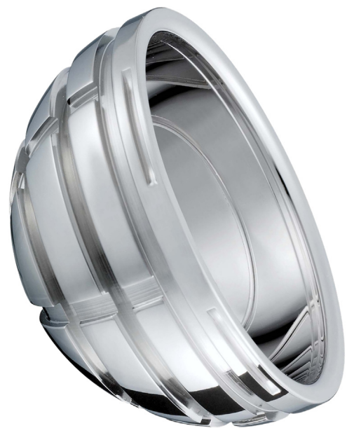
Fig. 1. Illustration of the Liberty AC (ATF, Marignier, France) dual mobility cup. The outer surface of the metal-shell is polished with concentric circumferential and radial grooves to improve cement interdigitation and cemented fixation strength.
