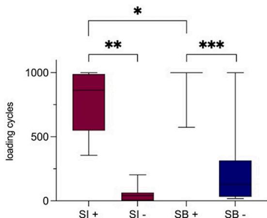
**Fig. 4.** graphic overview on the reached loading cycles. SI+ = SI-screws with anterior fixation, SI- = SI-screws without anterior fixation; SB+ = sacral bar with anterior fixation, SB- = sacral bar without anterior fixation. Comparison show statistical significant differences: \* SI+ vs. SB+  $p = 0.0238$ ; \*\* SI+ vs. SI-  $p = 0.0002$ ; \*\*\* SB+ vs. SB-  $p = 0.0014$ .
