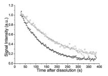
Figure 1. Decay curves of a two-compartment phantom. Both curves were normalized to their first point. The compartment without contrast agent (upper curve) had a relaxation time of  $181 \pm 8$  s, while the compartment with contrast agent decayed with  $T=99 \pm 2$  s.
