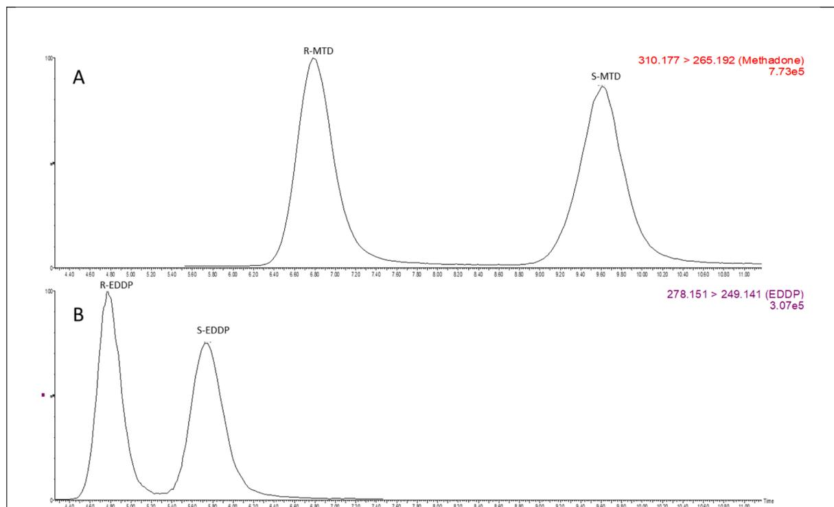
**Fig. 1.** Chiral LC separation using AGP column. Standards racemic mixtures were analysed at a concentration of 60 ng/mL. (A): R-methadone (RT: 6.78 min), S-methadone (RT: 9.61); (B): R-EDDP (RT: 4.77 min), S-EDDP (RT: 5.75 min).
