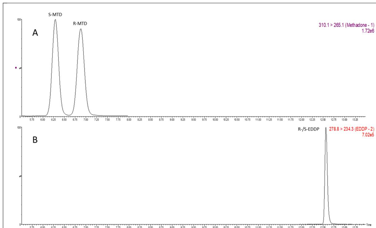
**Fig. 2.** Chiral SFC separation using Chiralpak IH-3 column. Standards racemic mixtures were analysed at a concentration of 60 ng/mL. (A): R-methadone (RT: 6.29 min), S-methadone (RT: 6.89); (B): R-/S-EDDP (RT: 12.57 min).
