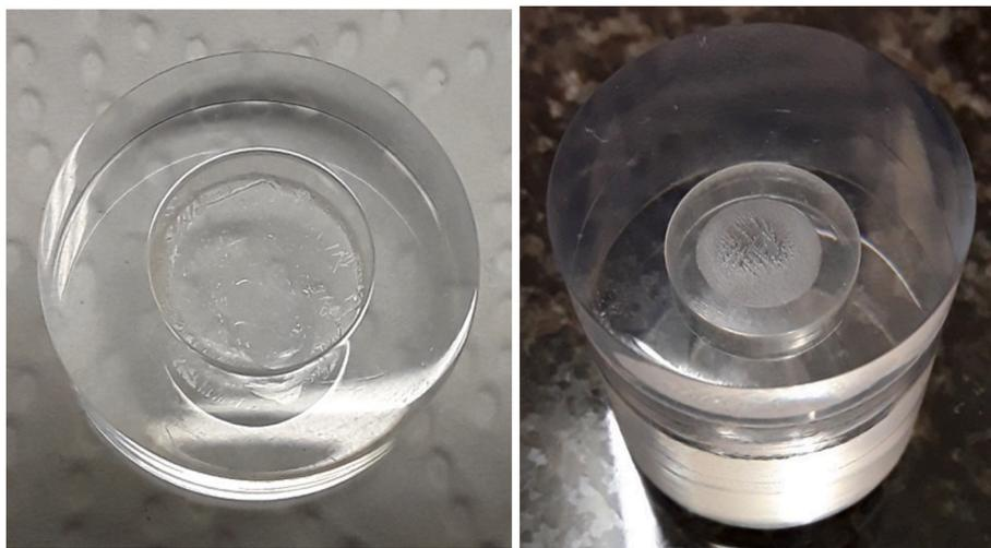
Fig. 1. UPS923A plastic scintillator with a crystallised  $^{32}\text{Si}$ - $^{60}\text{Co}$  deposit. Lanthanum nitrate and ammonium hydroxide were added on top of the liquid silicon and cobalt drops to prevent the volatility of silicon during drying.
