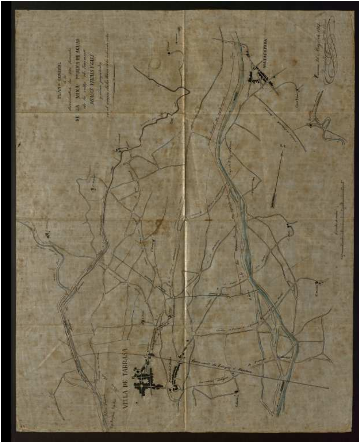
Figure 1.7. Map of the water mines planned and built by the water company to exploit the northern aquifer (1873). Note: the principal mine is represented by a tight blue line beginning in the village (bottom). The mine divides into the east (first fork) and the west (second fork). The planned mines are represented in red. Source: ACVOC-AHT, Collection ACVOC90-250 MPAT S.A., exp. UI P 47/34. Reprinted with the kind permission of the ACVOC-AHT.
