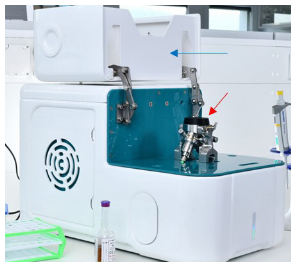
Figure 1 The red arrow points to the measurement head, visible and accessible for the operator. The measurement head and chamber are covered with a removable lid (blue arrow).
