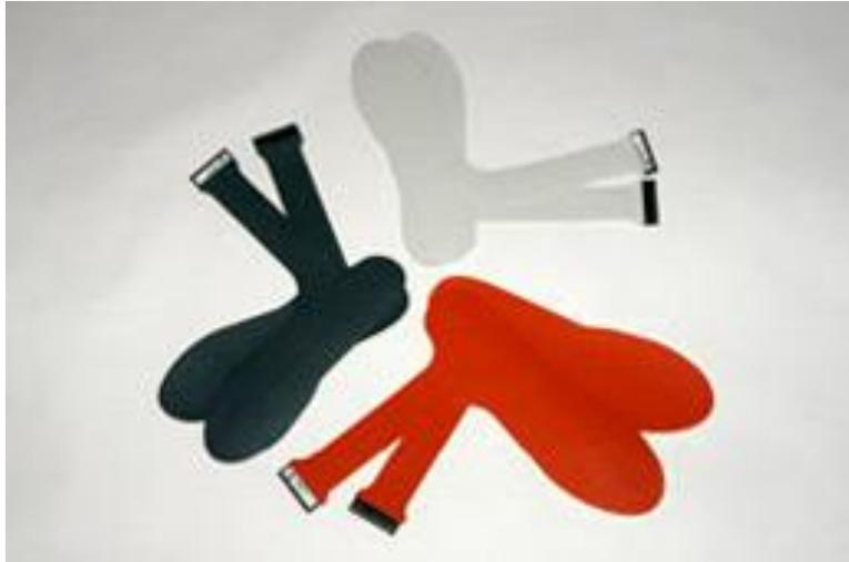
**Figure 8: Different PEDAR insole sizes.**
