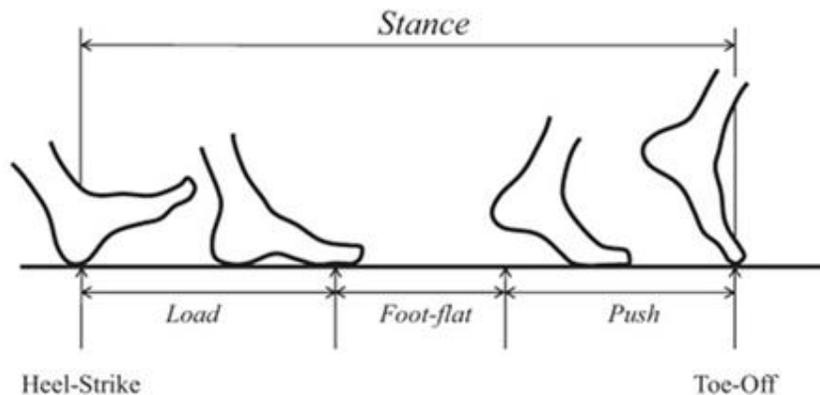
**Figure 10: Inner stance events showing load, foot-flat and push-off phases along with the heel-strike (initial contact) and toe-off (terminal contact). Image courtesy of B. Mariani [Mariani et al., 2013].**
