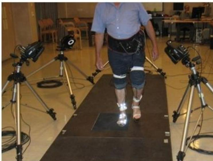
**Figure 6: Validation of utilized ambulatory gait assessment against the gold standard lab based method. Patient wearing inertial sensors and pressure insole, walking over the pressure plate embedded platform surrounded by high frame rate cameras. Image courtesy of H. Rouhani [Rouhani, 2010].**
