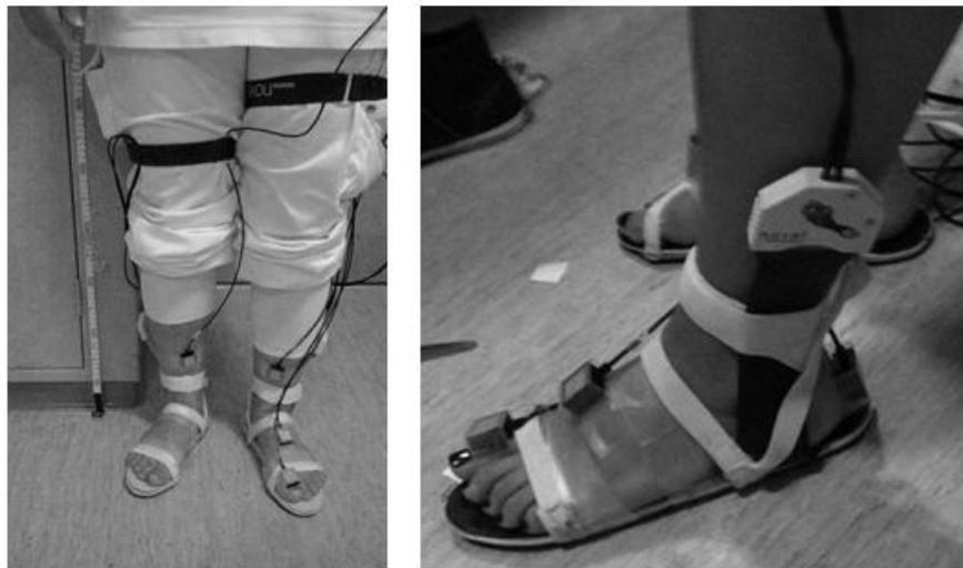
**Figure 7: Sensor placement for the ambulatory gait assessment system. On the tested ankle (left side) sensors are placed at the dorsal aspect of the proximal phalanx of the first toe, between the bases of the first and the second metatarsals, the great tuberosity of the calcaneus.**
