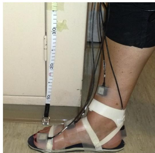
**Fig. 2.** Sensor placement for the tested foot.
