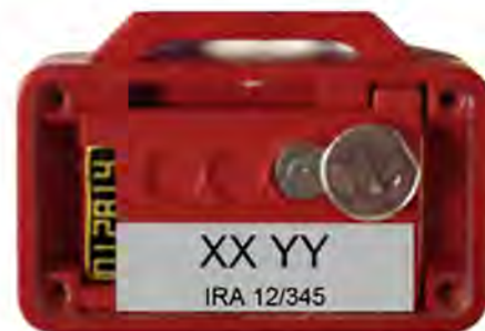
Fig. 1. Routine badge dosimeter used for this study, based on two TLD pellets.
