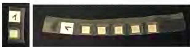
Fig. 2. Single TLD pellet in individual bag (left), TLD pellets in a plastic strip (right).
