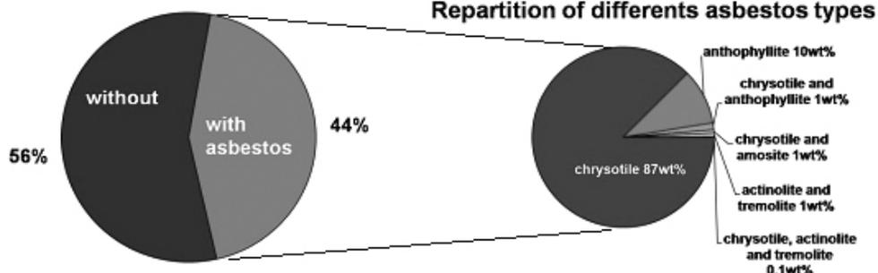
**Figure 1a.** Statistical repartition of approximately 10,000 different bulk building materials in Switzerland, analysed by the IST Laboratory of Mineralogy, 2000-2009.
