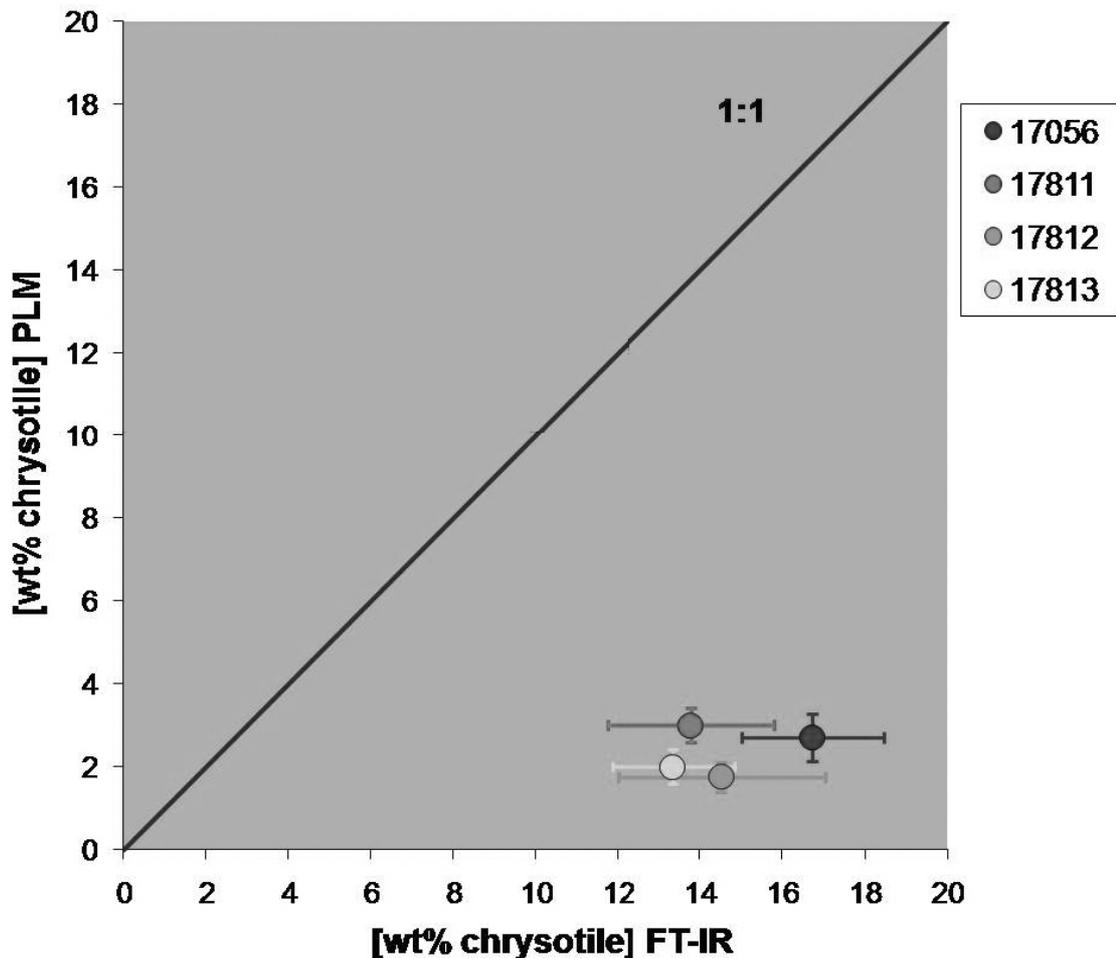
**Figure 2.** Comparison between 2 different methods of analysis: PLM versus FT-IR. *PLM*: all the samples are an average of 4 people's results. *FT-IR*: 17511, average of 5 results. 17056 and 17812, average of 6 results. 17813, average of 21 results.
