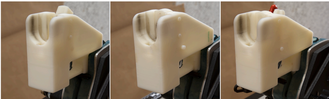
Fig. A3. Z-ABS Liberators printed with an infill density of 100% on the Zortrax M200 (ME).
