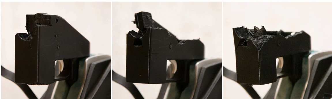
Fig. A4. Z-PETG Liberators printed with an infill density of 70% on the Zortrax M200 (ME).
