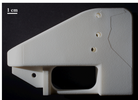
Fig. 8. One of the frames printed with the PBF printer, the incompleteness of the last layer can be seen on the right.
