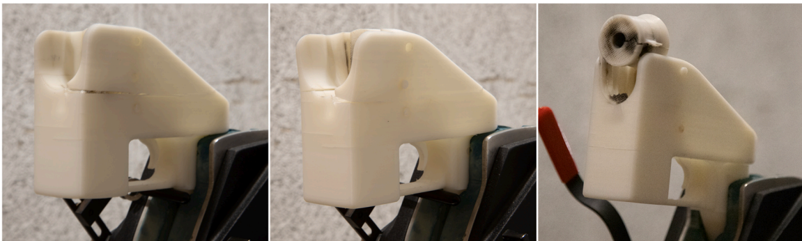
Fig. A2. Z-ABS Liberators printed with an infill density of 70% on the Zortrax M200 (ME).
