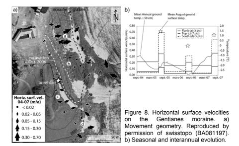
Following the excavation of October 2006 (cf. Fig. 8a), the measurement of 30 new blocks located on the road was carried out in order to follow the readjustment speed of the active layer. In one
