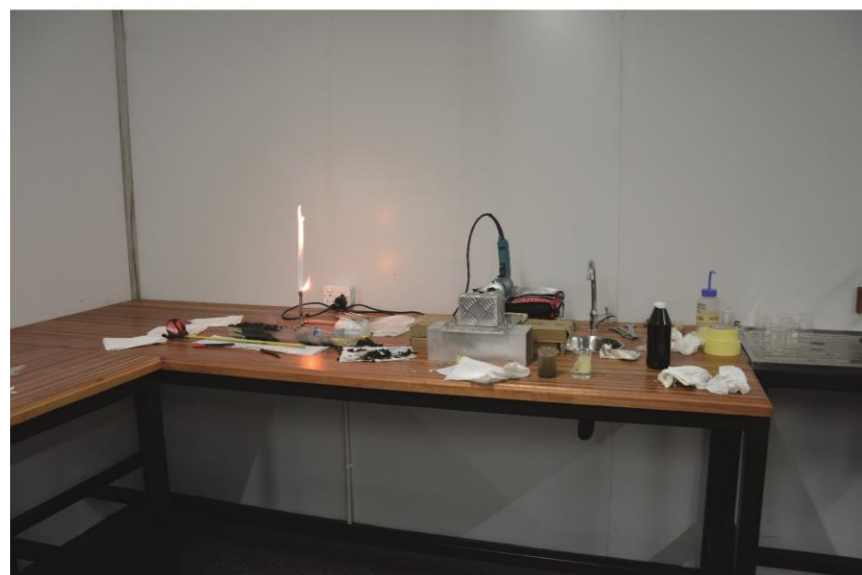
VanThuyne-Ridge Research Center March 2017 Work table for opening and segmenting cores from Lake Liambezi in a controlled atmosphere and sterilized equipment for samples dedicated to microbiological and sedimentary analyses.
