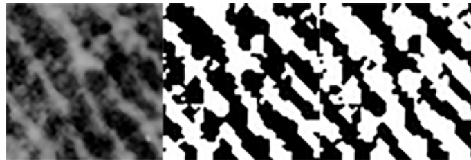
Figure 2-1: The image on the left represents the original ROI (the darker color pixels correspond to friction ridges). The image in the center represents the binary mask of the segmented ROI for which the black areas correspond to pixels thresholded as “signal.” The image on the right represents the binary mask of the segmented ROI for which the black areas correspond to pixels thresholded as “background” (i.e. the image on the right is the inverse of the image in the center). NOTE: Actual size of images are 2.54mm x 2.54mm. Images are enlarged and pixels interpolated for illustration.
