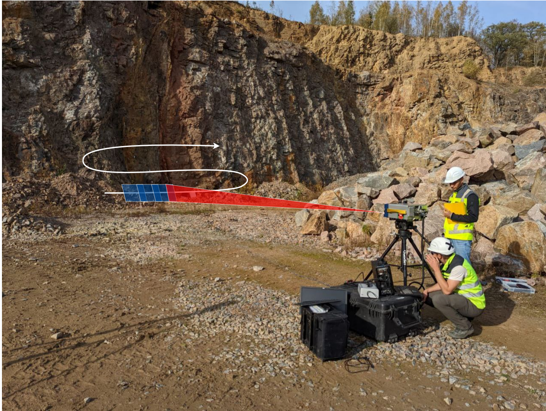
Figure 4.2: Target wall and imaging procedure: the images (blue squares) were taken as to make a snake shape (white arrow)
