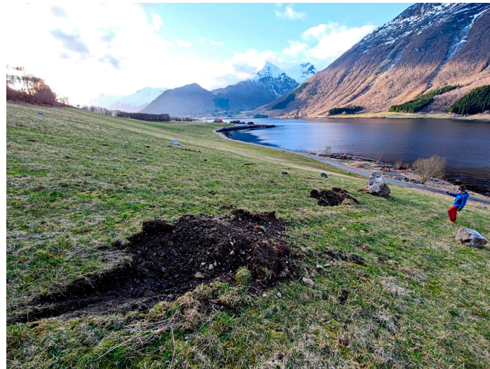
Figure A9. Example of an impact scar observed in the field. Note how clearly defined is the entry point of the scar compared to the exit point. As a side note, small rockfalls that occur in fields are likely to be removed by landowners, thus affecting onsite data collection.
