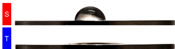
Fig. 1. Water wettability of Nitinol disks: Standard (S, top) and treated (T, bottom) disks with a water droplet placed on the center.
