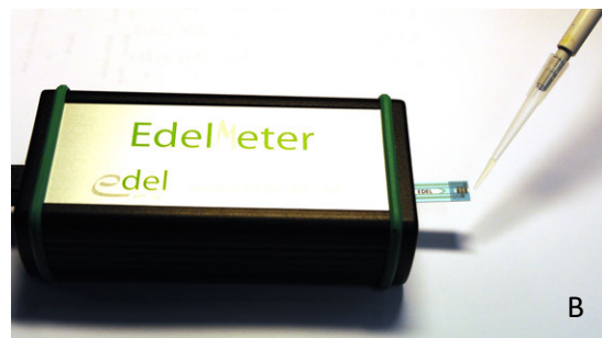
Figure 2 – Electrochemical measurement of antioxidants with the Edel technology. [A] Illustration of the electrochemical sensor, workstation as well as the output signal. [B] Illustration of sample loading. AO: antioxidant, I: current in ampere (A), E: potential in volt (V).
