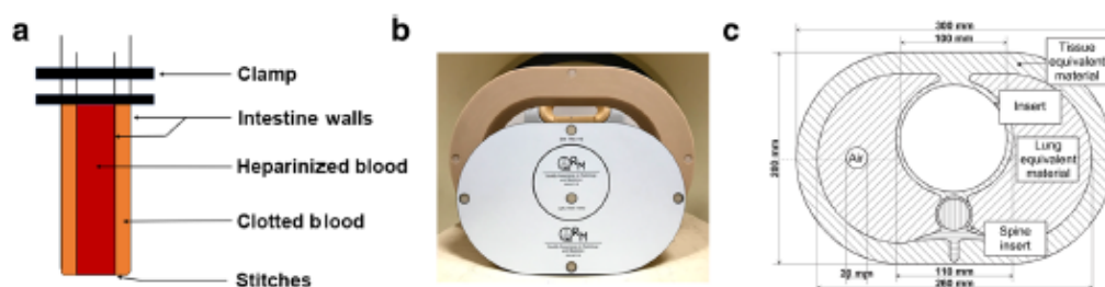
Fig. 1 Representation of the aortic intramural hematoma (a) and anthropomorphic (b, c) phantoms. The false and inner lumen were filled with blood with extra iodinated contrast media for the inner
