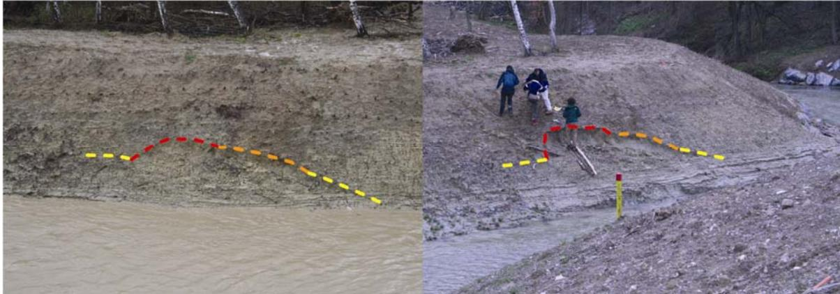
Figure 6: Photographs of the second landslide (left: taken on 10<sup>th</sup> of April 2006 during the flooding; right: situation on April 12<sup>th</sup> 2006). The main scarp (red), the secondary scarp (orange) and the minor scarps (yellow) are discernable on both pictures. The landslide continued its rotational movement in the interval of the two pictures.
