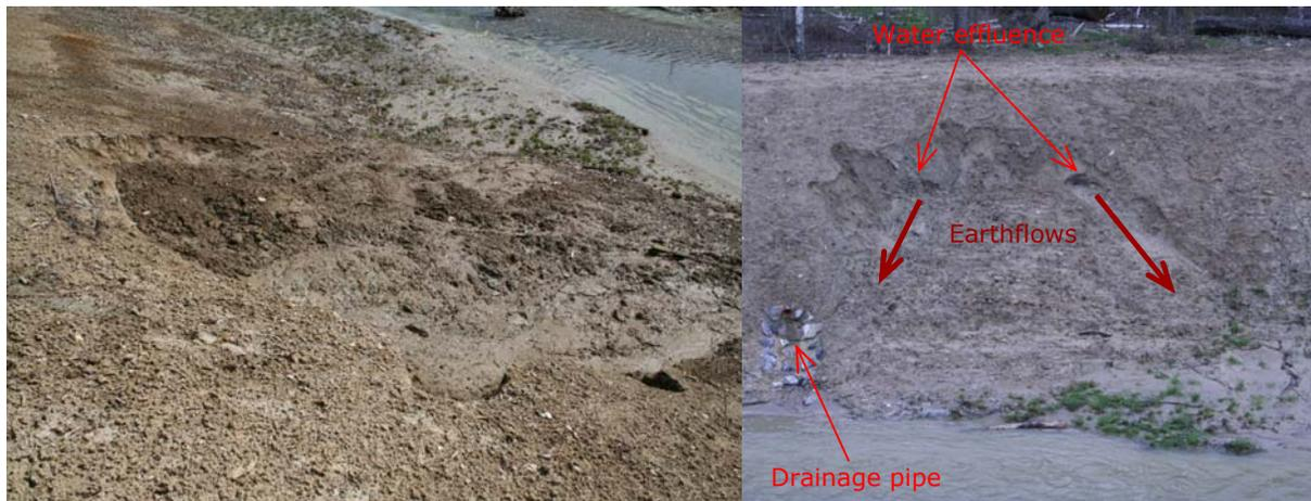
Figure 2: Photographs of the pre-existing landslide (left: taken on March 16<sup>th</sup> 2006; right: taken on April 12<sup>th</sup> 2006). The circular failure surface, the landslide's head and foot are visible. The main body of the slide is wet, indicating arrival of groundwater. Water effluences are observable on the picture taken on April 12<sup>th</sup> 2006. They probably caused some small earthflows.
