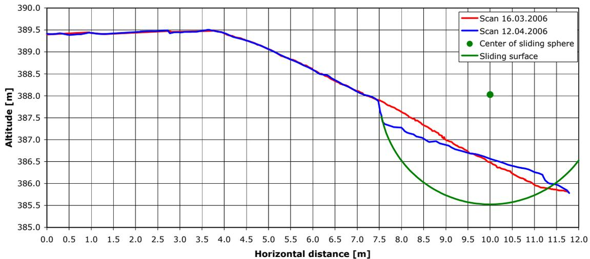
Figure 8: Cross section through the second landslide. The scan made on March 16<sup>th</sup> 2006 shows no traces of potential landsliding (red line). The scan of April 12<sup>th</sup> 2006 (blue line) shows the rotational displacement of the initial planar surface. The trace and centre of the sphere (in green) is fitted using the points of the main scar and represents the sliding surface.
