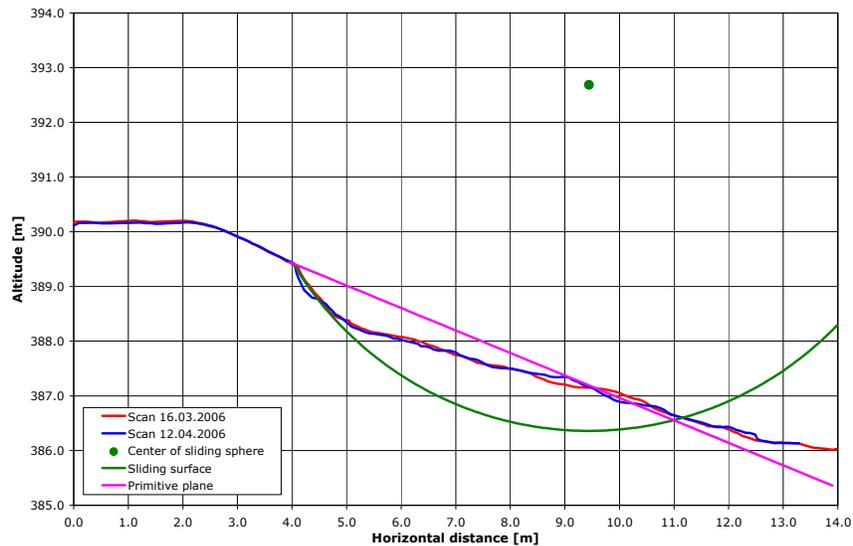
Figure 5: Cross section through the first landslide. The differences between the two scans (red: March 16<sup>th</sup> 2006; blue: April 12<sup>th</sup> 2006) are caused by the minor slides in the scar area and the earthflows. The trace of the primitive plane corresponding to the initial surface (in pink) is shown. The best-fit sphere and its centre (in green) represent the sliding surface and the rotation axis.
