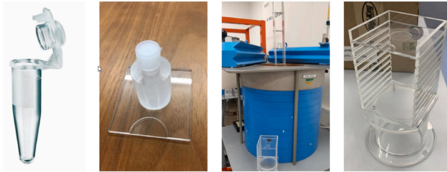
Fig. 10. Images from the source container, positioning system and detector enclosure at UniBern. From left to right: Eppendorf vial, bottle where the Eppendorf vial is inserted, detector enclosure and methacrylate positioning device.
