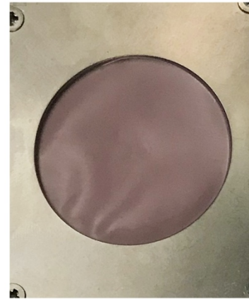
Silicone disk sandwiched between one stainless steel plate and one plastic piece (with a teflon disk between silicone and plastic)
