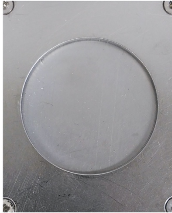
Silicone disk sandwiched between two stainless steel plates
