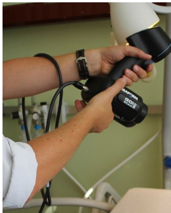
Fig. 1. Surface acquisition. Surface acquisition with the surface scanner.
