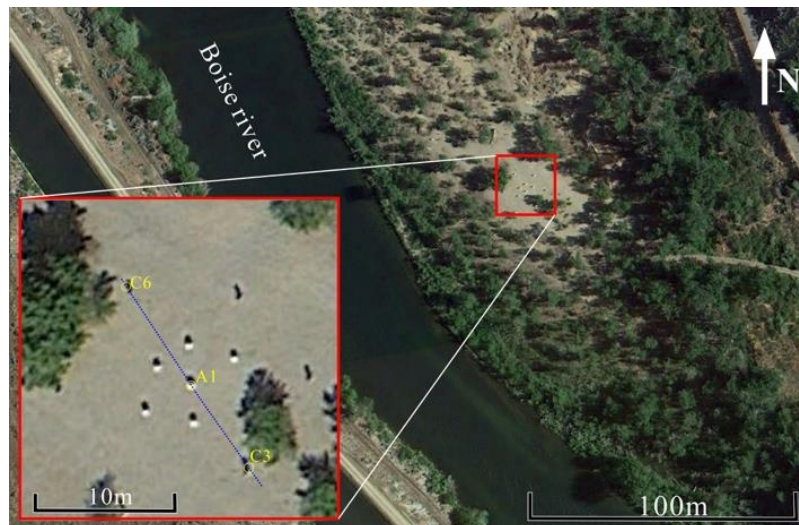
Figure A.7: Location of BHRS wellfield in relation to the Boise River. The dashed blue line joining wells C6, A1, and C3 corresponds to the considered surface-based GPR reflection survey.
