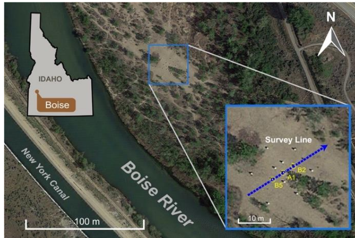
Figure 3.11: Map of the BHRS ( 43^{\circ}32'32'' N, 116^{\circ}05'52'' W) showing the location of the considered common-offset GPR reflection profile (blue dashed line). The profile is aligned with boreholes B5, A1, and B2 (yellow circles).
