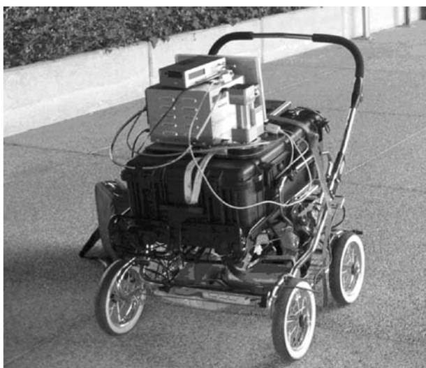
**Fig. 1.** Transport system used to make the WRAS (consisting of an SMPS, portable aerosol spectrometer, and laptop computer) more mobile.
