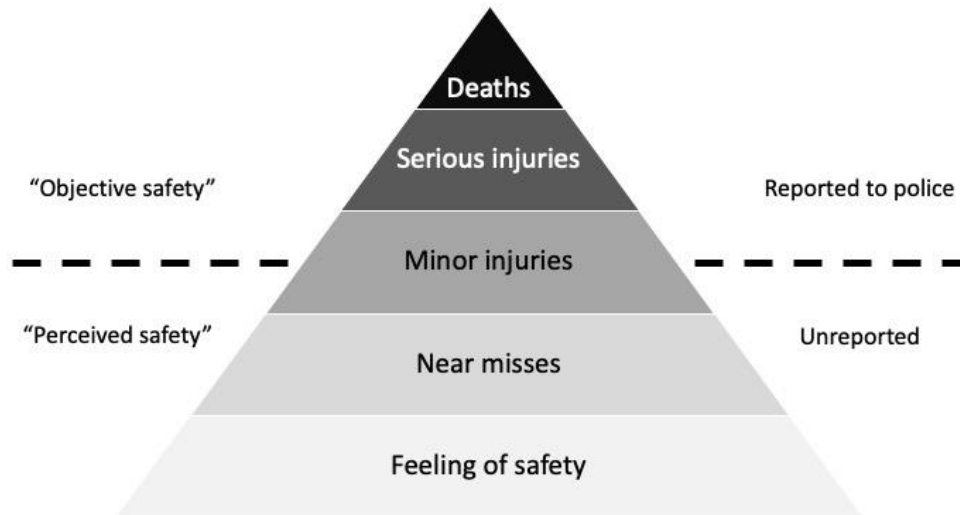
Figure 8: The Heinrich Safety Triangle, or crashes as the "tip of the iceberg" of cycling safety. Adapted from Hamann & Peek-Asa (2017).
