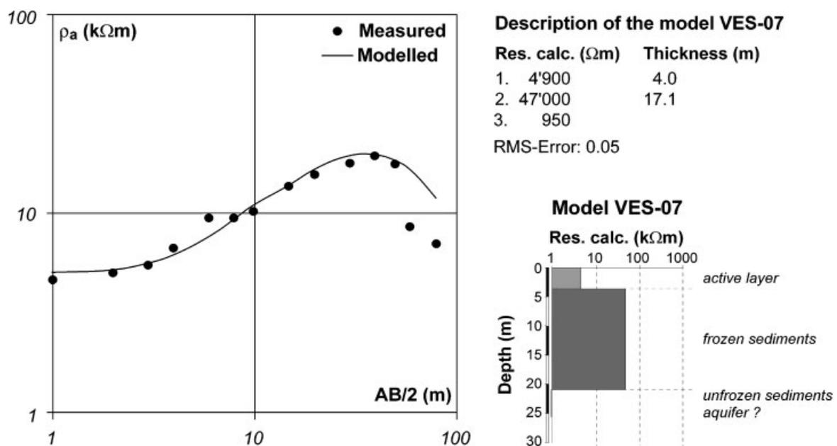
Figure 2 Curve and interpretation model of the VES-07 (vertical electrical sounding) carried out longitudinally on the centre of the rock glacier (see Figure 1 for the VES position).
