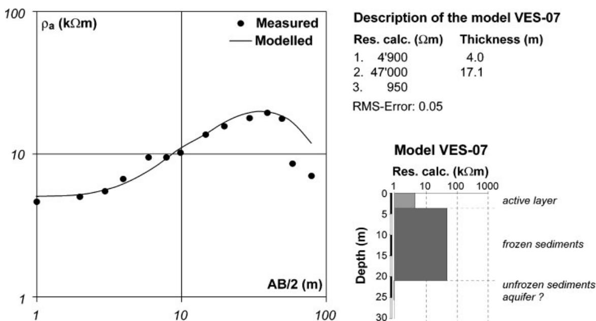
Figure 2 Curve and interpretation model of the VES-07 (vertical electrical sounding) carried out longitudinally on the centre of the rock glacier (see Figure 1 for the VES position).
