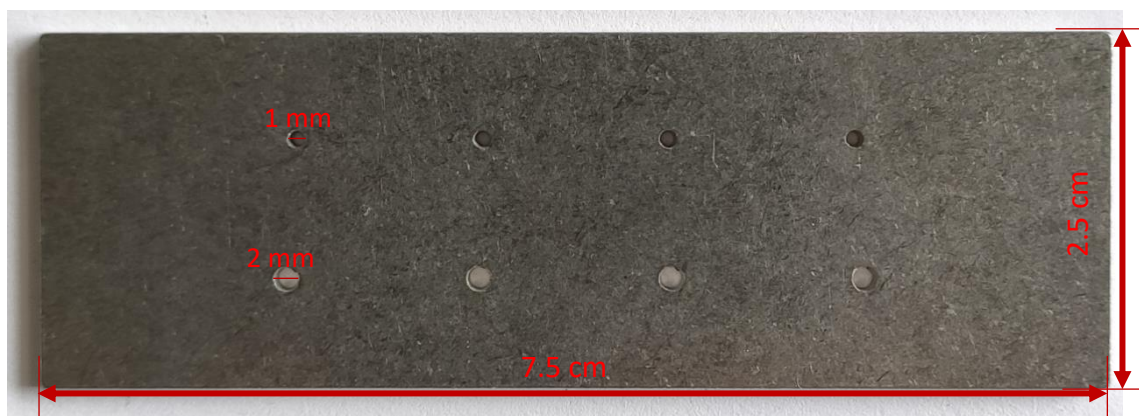
Figure 31. A custom-made steel stage for no support sample preparation.
