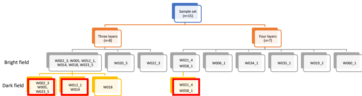
Figure 26. Classification of the select sample set using transmitted light bright field and dark field. Red boxes indicate the undifferentiated pairs.
