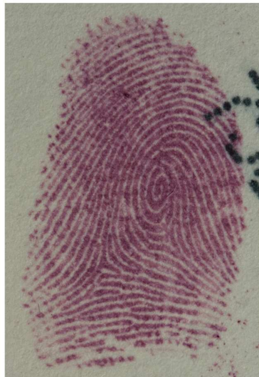
(Left) Molecular representation of Ninhydrin (2,2-dihydroxy-1,3-indanedione); (Right) Representative fingermark detected using this technique (paper as substrate).
