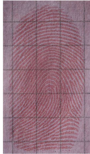
(Left) Molecular representation of Oil Red O; (Right) Representative fingerprint detected using this technique (paper as substrate). 109x61mm (400 x 400 DPI)
