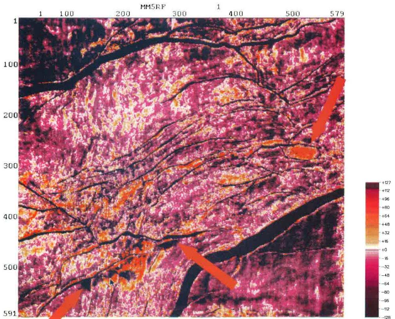
Fig. 6-12: Amplitude map along the MM5-44 horizon (NE-SW reworked sand bodies and bright spots).
