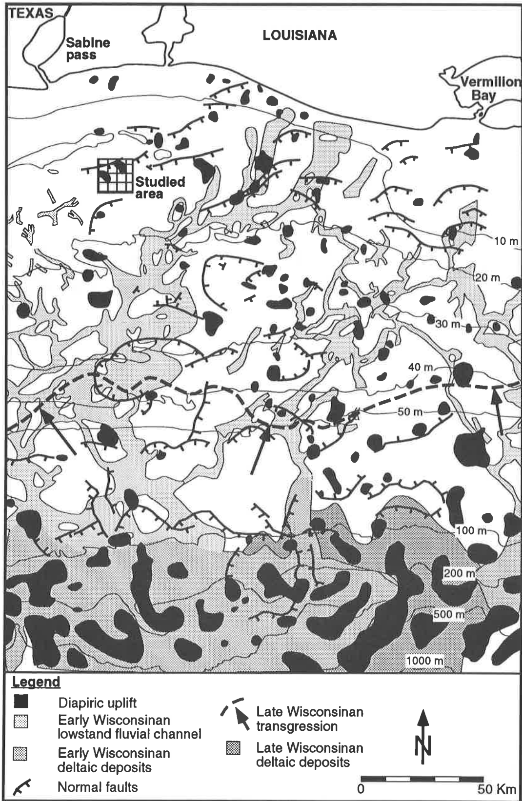
Fig. 5-5: Early and Late Wisconsinian erosional streams and deltaic systems and line of maximum of Late Wisc. transgression superposed on salt and fault related morphology of the offshore Louisiana portion of the Gulf coast shelf. True scale studied area is indicated.
