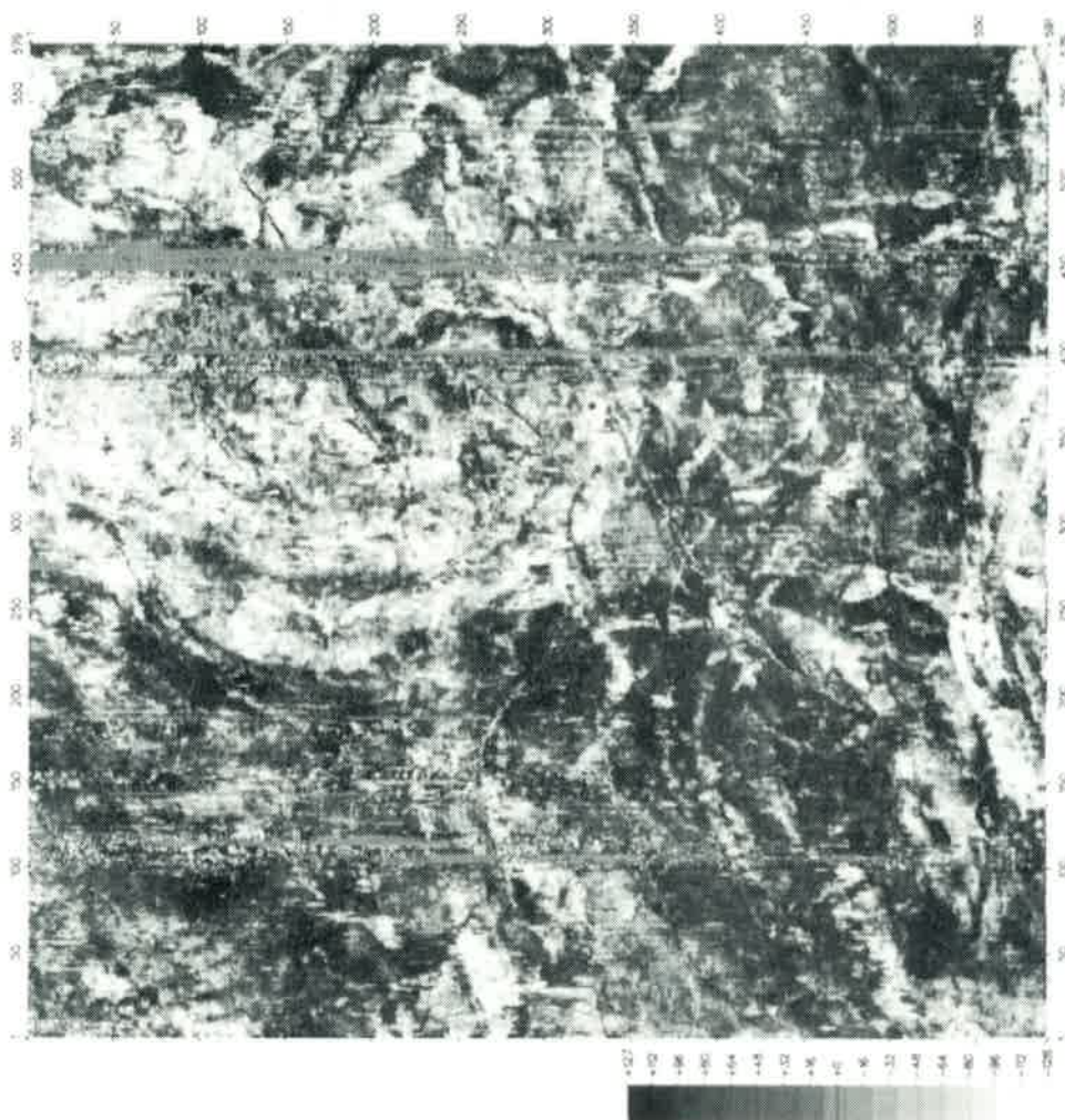
Fig. 5-39: c. Drastic change in seismic facies 4 ms above LATEPLIO-44 showing the base of highstand delta lobe progradation towards the SW.
