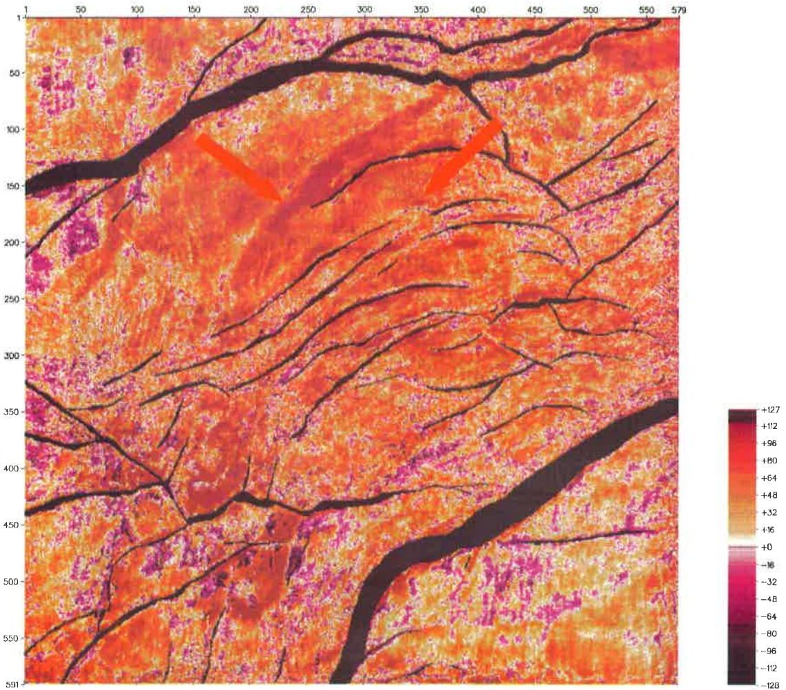
Fig. 6-11: a. Amplitude map calculated 20 ms below the MM5 horizon (NE-SW channel and fan).
