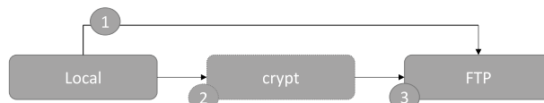
Fig. 7. Comparison of directly using a remote FTP (1) vs. using a virtual crypt remote (2) which then will access the actual FTP remote (3).
