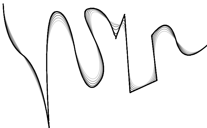
Figure 4.3: A 2D curve (in black) along with its smoothed versions (in gray) for increasing values of the smoothing factor \sigma . It is appreciable how the smoothing affects the shape of the signature, in particular by reducing the total length.
