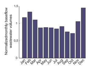
Figure 1. Monthly variations of dry weather flow at the Vidy Bay WTP inlet. Flow is normalized to the annual mean flow, which is  $18\times10^6\,$  m³. The monthly baseflow fluctuates between +40/-25% of the mean.
