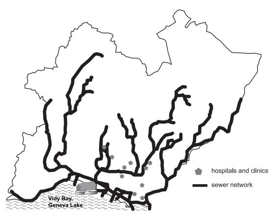
**Figure 2. Schematic view of the Vidy Bay WTP basin considered in this study.** The main pipes of the collection system are illustrated with bold lines. Hospitals and clinics for acute somatic treatment are located using grey pentagons. The total number of hospital beds in the basin is about 1600, which corresponds to a total of approximately 8 beds per 1000 inhabitant. doi:10.1371/journal.pone.0053592.g002
