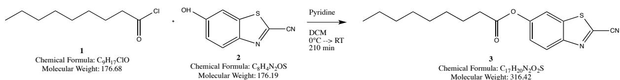
Figure 5-0-2 Synthesis of C<sub>9</sub>-CBT (Toya, Y. et al., Bull. Chem. Soc. Jpn, 65, 2604-2610 (1992))
